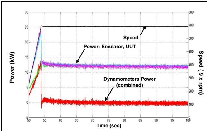
**Figure 10:** Test Results (Component power output at 6000rpm, 20Nm)
