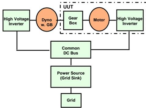
Figure 2: Common DC bus system
