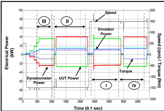
**Figure 7:** Test Results (Component electrical power in four quadrants)
