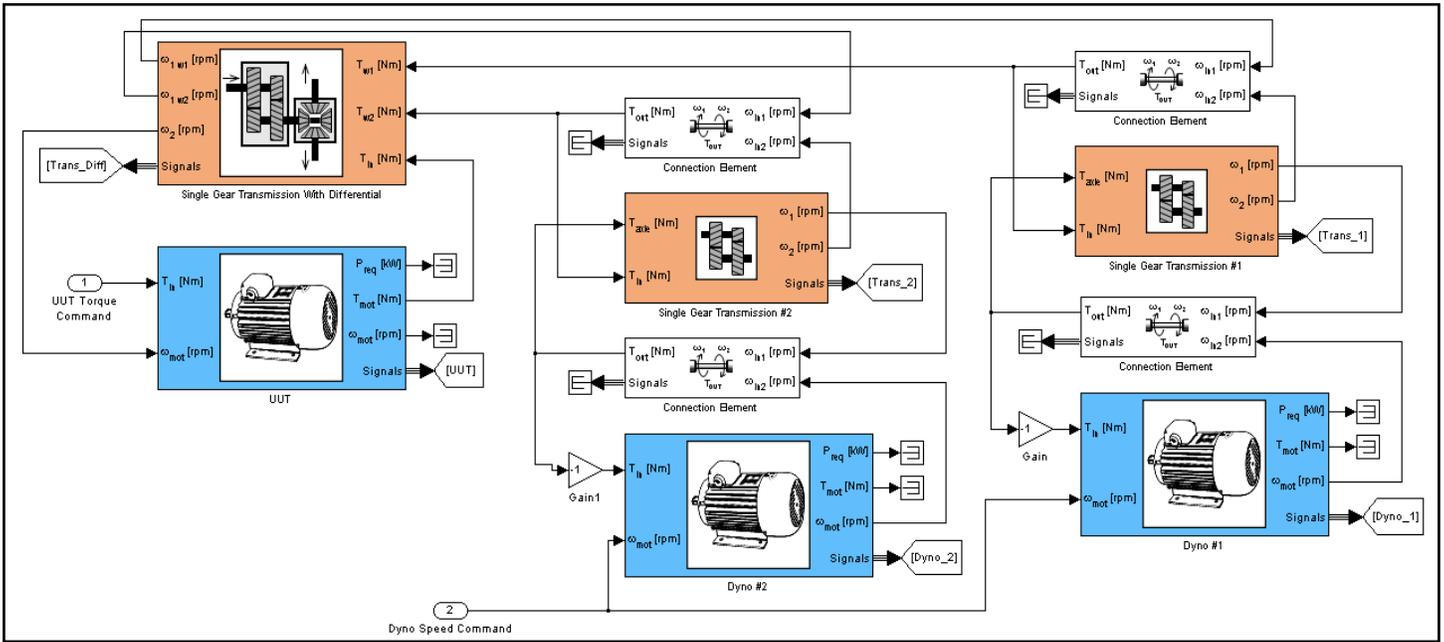
Figure 5 : Test Cell Simulation Block Diagram
