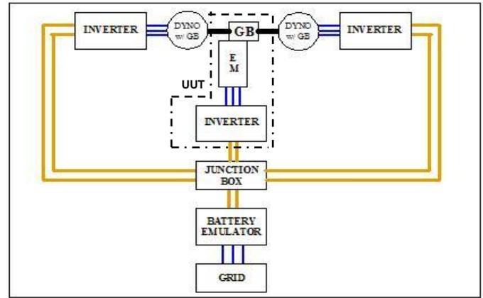
Figure 4: Common DC Bus FR EPT Drive Test Bench
