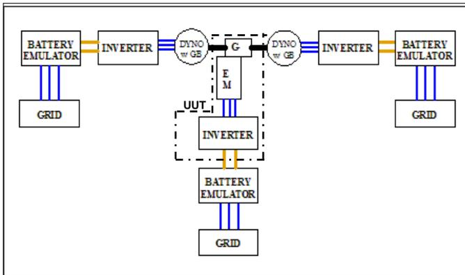
Figure 3: Separate DC Bus FR EPT Drive Test Bench
