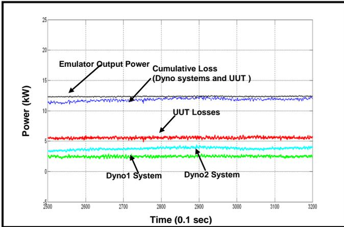
**Figure 9:** Test Results (Component electrical power at 1500rpm, 200Nm)
