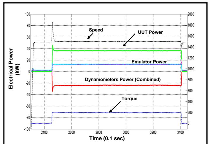
**Figure 8:** Test Results (Component power losses at 1500rpm, 200Nm)
