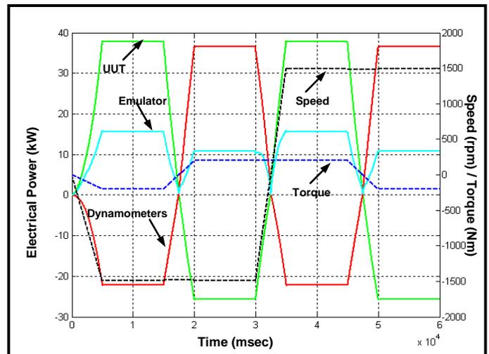
Figure 6: Simulated power requirements of UUT and dynamometers
