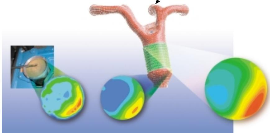
Concurrently, the available volume for the converter is restricted by reduced packaging area. Furthermore, the exhaust flow needs to sweep the catalyst as uniformly as possible to guarantee optimum conversion of pollutants.
