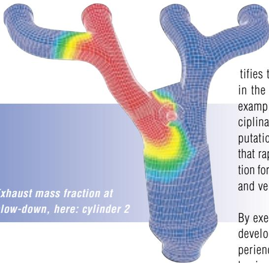
Exhaust mass fraction at blow-down, here: cylinder 2
