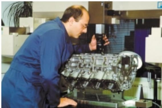
Coordinate Measuring Maschine
