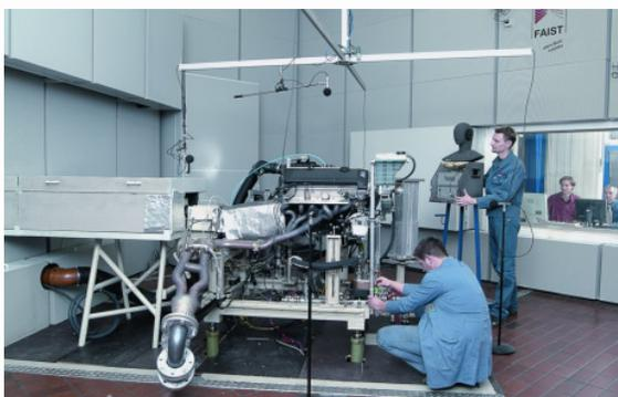
Fully equipped NVH test bench incl. test object
