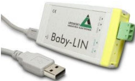
The Baby-LIN allows to control LIN-bus equipped devices by use of an off the shelf standard personal computer. The only requirement is an USB-port on the PC.
