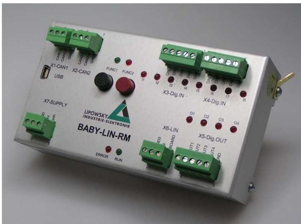
The Baby-LIN-RM allows to control LIN-bus equipped devices by use of an off the shelf standard personal computer. The only requirement is an USB-port on the PC. Furthermore LIN devices can be controlled by simple digital i/o signals.
