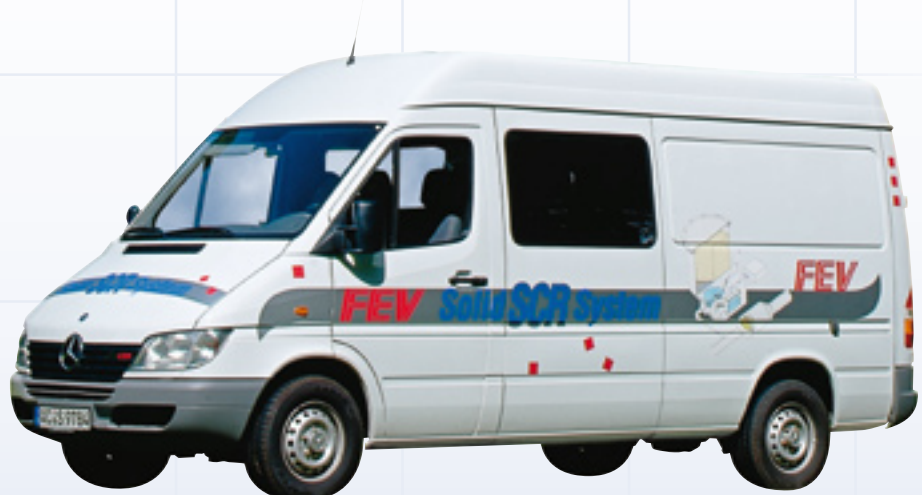
LDV Demonstrator Vehicle with FEV Solid SCR System based on ammonia carbamate
