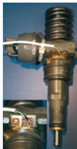
Injection Pressure Measurement with Strain Gauges
